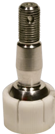
Non-serviceable plastic design has failed due to intrusion and wear.
